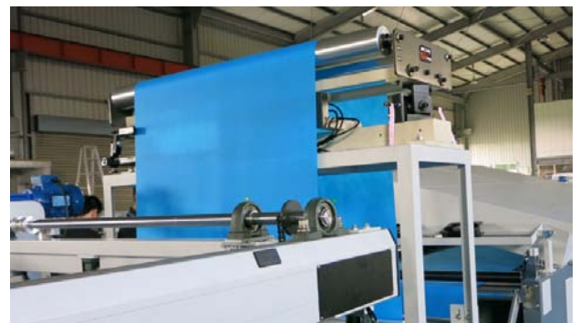
Center Pivot Guider C-1300-JF is used on a Screen Printing Machine
